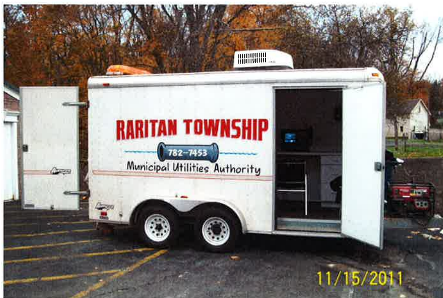
Photo No. 2 – CCTV equipment trailer and monitoring station. Inspection services arranged with Raritan Township MUA
