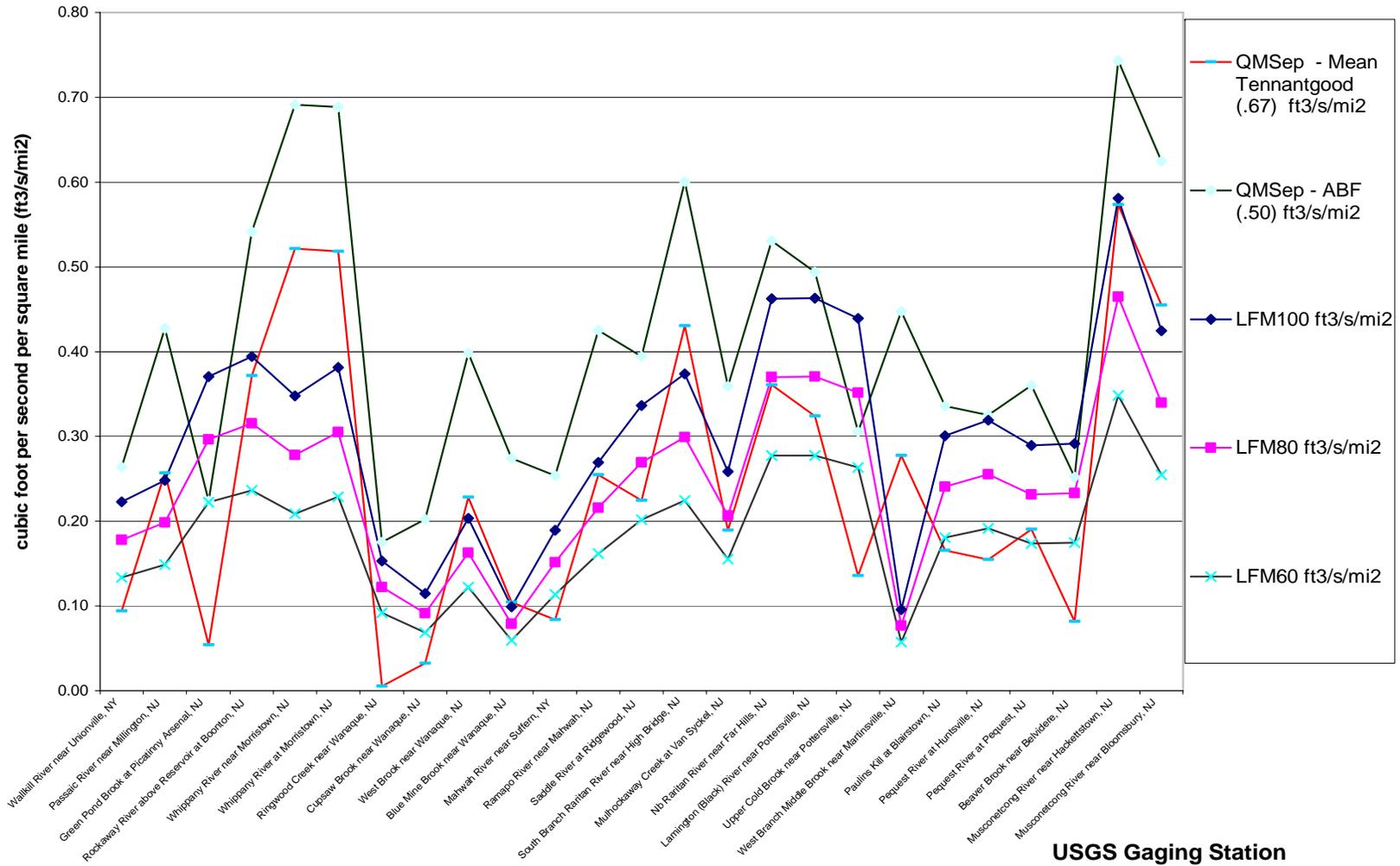
Figure 1: Comparison of estimates of water capacity using a variety of stream flow statistics (Tennant, Aquatic Base Flow and Low Flow Margin at 100%, 80% and 60%). Note: Low Flow method (LFM) values do not reflect reductions due to consumptive/depletive uses at full allocation.
